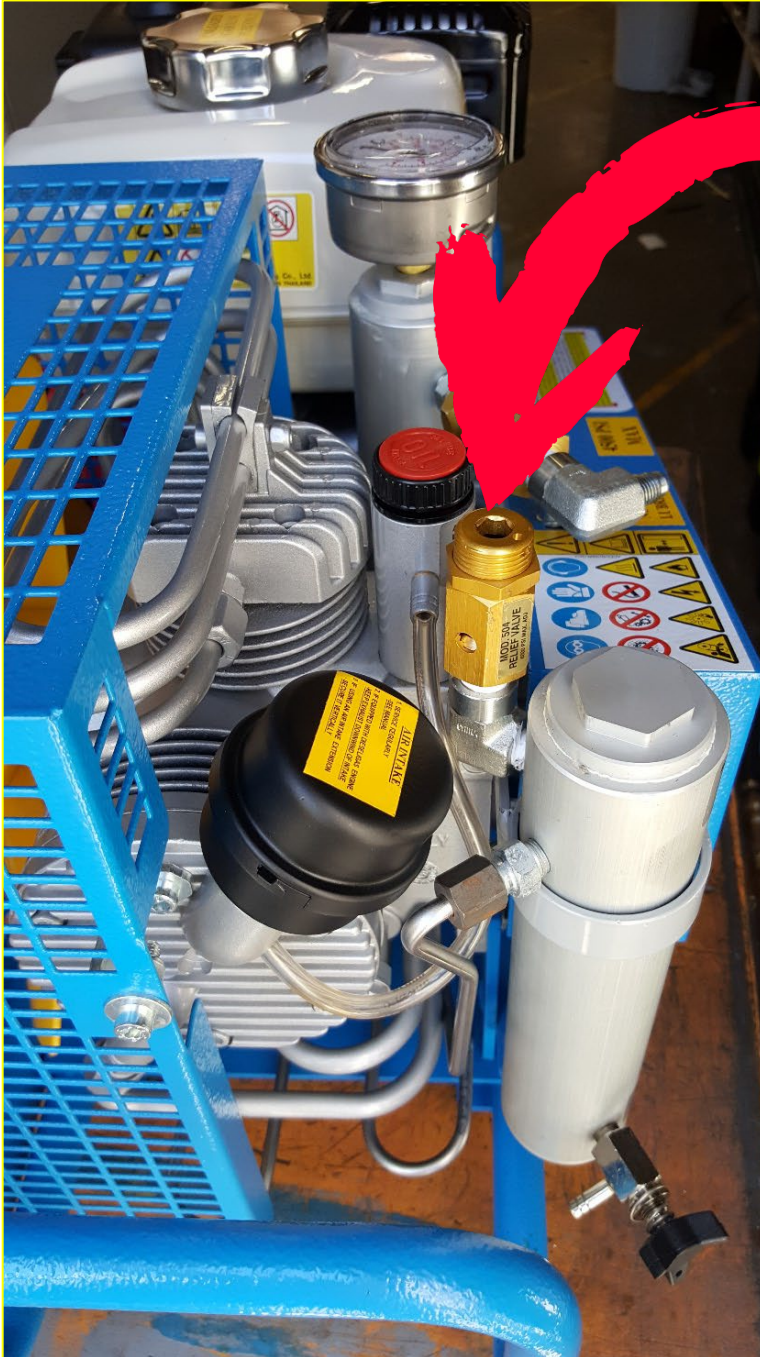
Pictured: Main overpressure (OP) relief valve as seen on MCH6 compressor.
