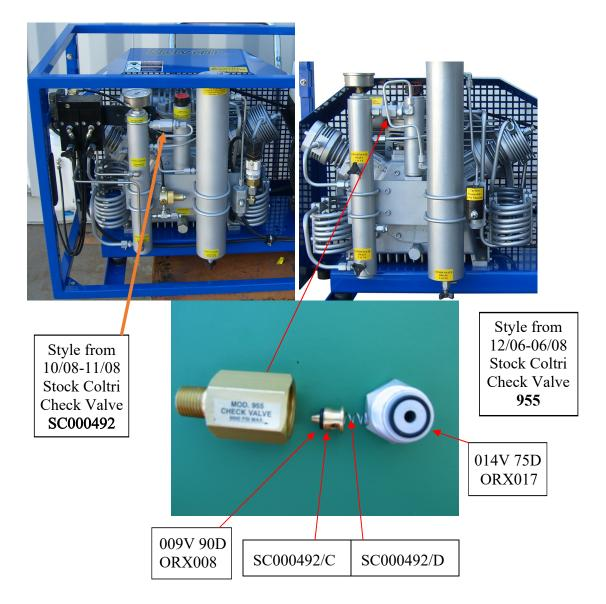
The check valve on the left is not the same as the 955 valve on right!
