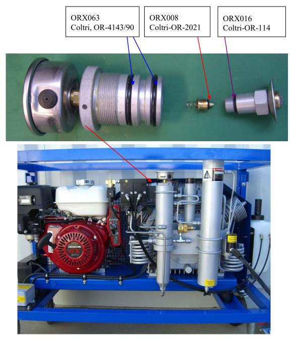
Open all manual drains while performing service! Do not hand twist gage to remove cap! Replace ORX008 if air is leaking from auto drain when compressor is not running.
