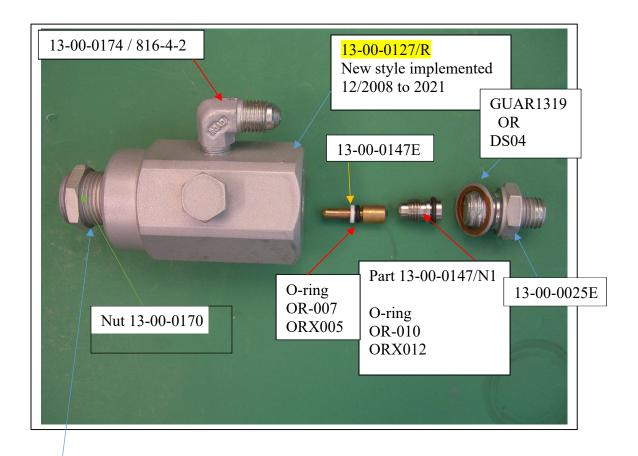
The pressure maintaining valve needs to be tested and or reset after assemble. Failure to set the valve, may lead to death, sever injury and catastrophic compressor failure.
