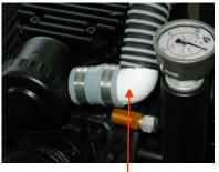
Secure hose to nitrox compressor intake with hose clamp as shown on this Coltri HP compressor.
