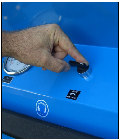
Step 20: Close fill station door.
