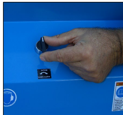
Step 3: Open front door by turning door switch. Door opens automatically.
