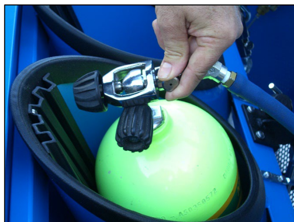
Step 16: Open fill whip bleed valve to relieve pressure.
