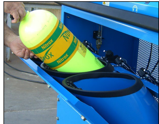
Step 5: Place cylinder into fill containment station compartment.
