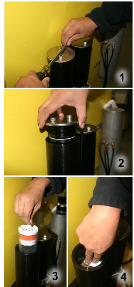
Figure 6. Changing air filter cartridge.
