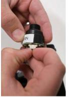
Step 5. Remove Old Sensor from Case by Unscrewing
