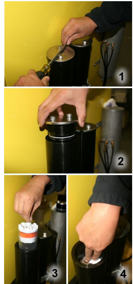
Figure 21. Changing air filter cartridge.
