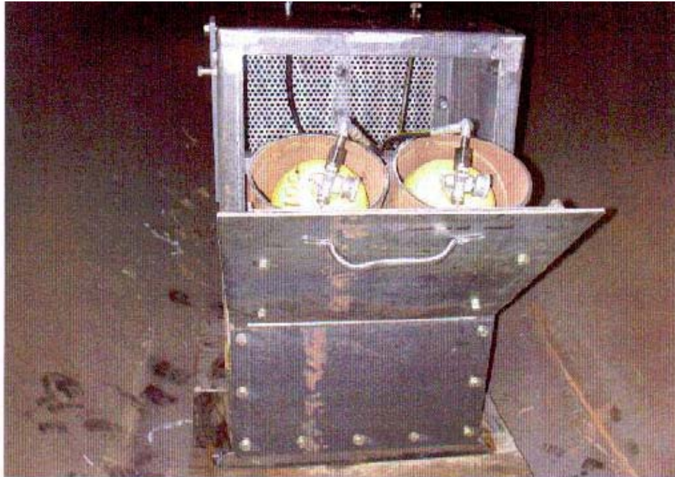
Figure 1: 2 cylinder enclosure before cylinder rupture
